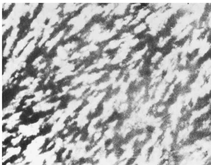
FIGURE 16 Microstructure of \beta -naphthol- m -aminophenol eutectic I, \times 50 (high velocity).
