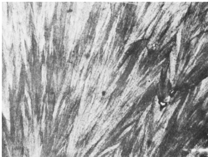
FIGURE 23 Microstructure of \alpha -naphthol- \beta -naphthol-phenanthrene eutectic, \times 50 .
