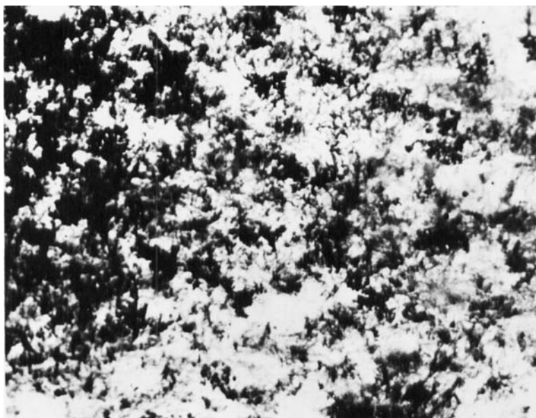
FIGURE 14 Microstructure of \beta -naphthol-phenanthrene eutectic, \times 50 .
