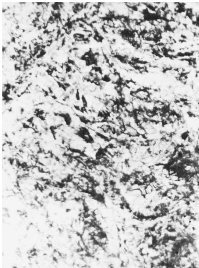
FIGURE 26 Microstructure of \alpha -naphthol- \beta -naphthol- m -aminophenol peritectic. X50.
